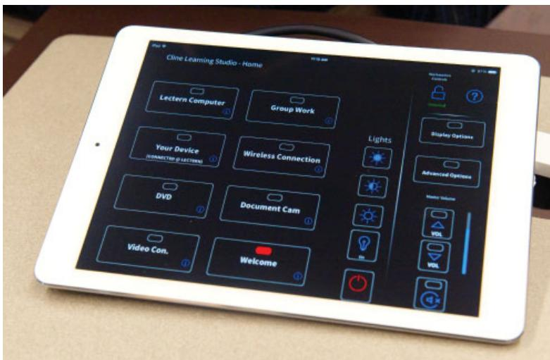
Crestron touch screen built into the podium, or from an iPad® equipped with the Crestron app.
