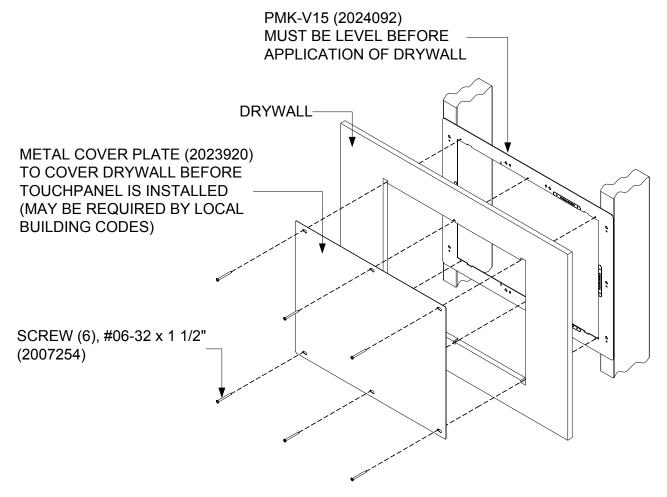
**NOTE:** MOUNTING PLATE IS TO BE COVERED WITH DRYWALL AND THEN THE CUTOUT MADE AROUND THE INSIDE OF THE OPENING.
