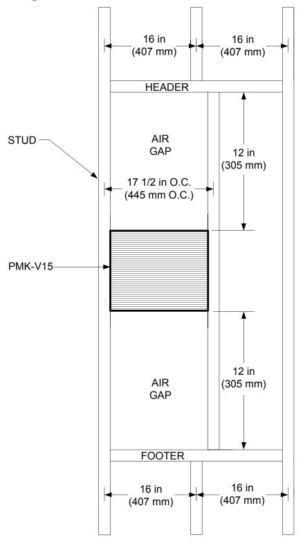
2. Using the level, attach the PMK-V15 to both the left and right studs using drywall screws or nails (not included). Make sure that the mounting kit is attached to the center of the studs. Refer to the image below for visual guidance.
