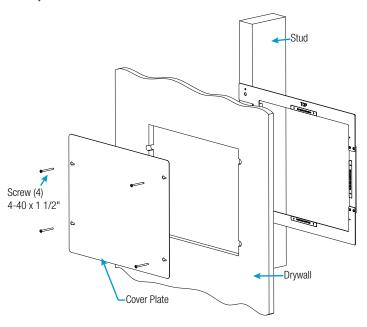
**NOTE**: The four tapped holes on the front of the mounting plate must be exposed to accept the docking station's mounting screws. The holes are found beneath the drywall just outside the four corners of the drywall opening.
