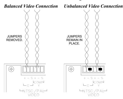
If there is no video signal, do not make a connection to the port, but leave the connector with the jumpers attached to the NTSC/PAL VIDEO sixposition mini-terminal block connector on the TPS-IMW.
