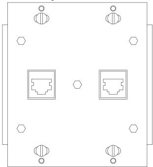
Once the TPS-IMW is installed into a 2-gang electrical box, it can be covered with a Decora wallplate (purchased separately).
