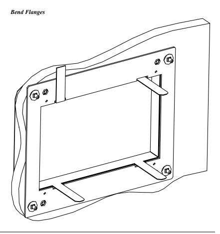
**NOTE:** The mounting plate will have a little play; this is normal. It allows for minor adjustments to the touchpanel during installation.
