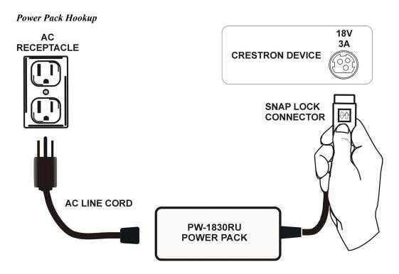
**NOTE:** Pull back the snap lock portion of the power supply connector to unlock it from the input when removing the connector.
