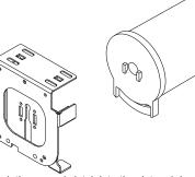
4. Push the manual clutch into the slot and down to engage the tabs. Secure the Manual Clutch to the Manual Clutch Bracket.
