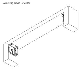
For a recessed or extruded pocket, the tab on the manual clutch-side bracket must be removed to install the shade. It is not necessary to reattach the tab after the shade is installed.
