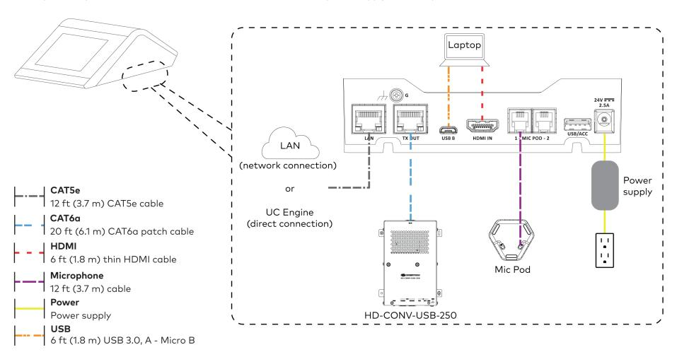
3. Connect the power supply and camera to the bottom of the content ingest device (HD-CONV-USB-250). Connect the power supplies to an AC power outlet.
