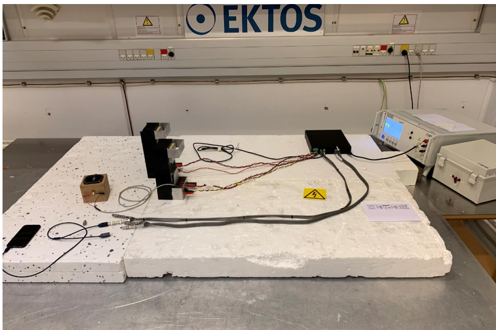
Photo 14. Voltage dips and interruptions test setup.
