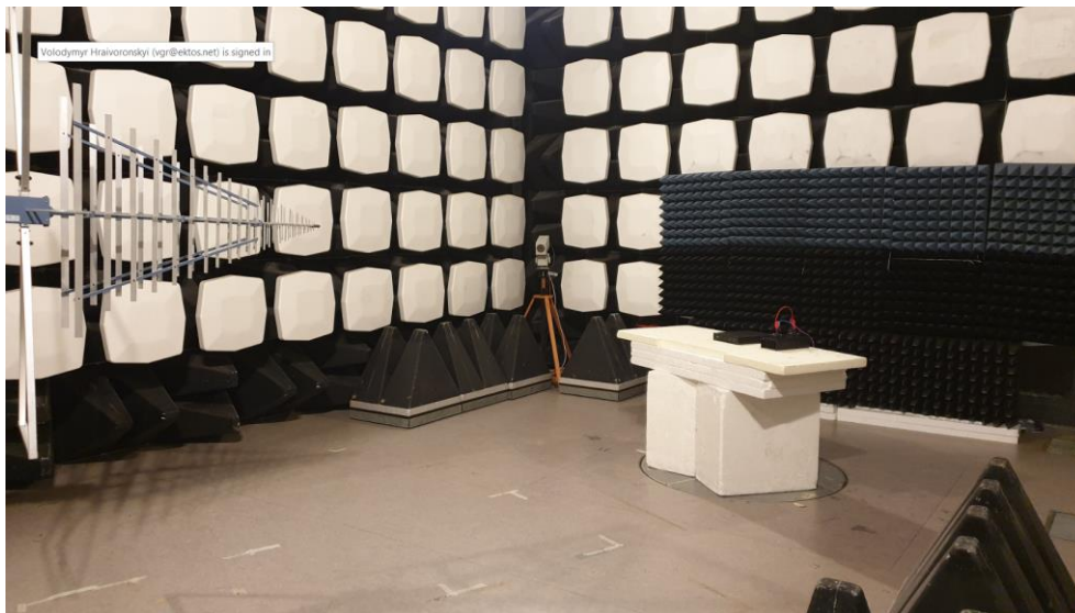
Photo 3. Radiated emission test setup. 30 - 1000 MHz.
