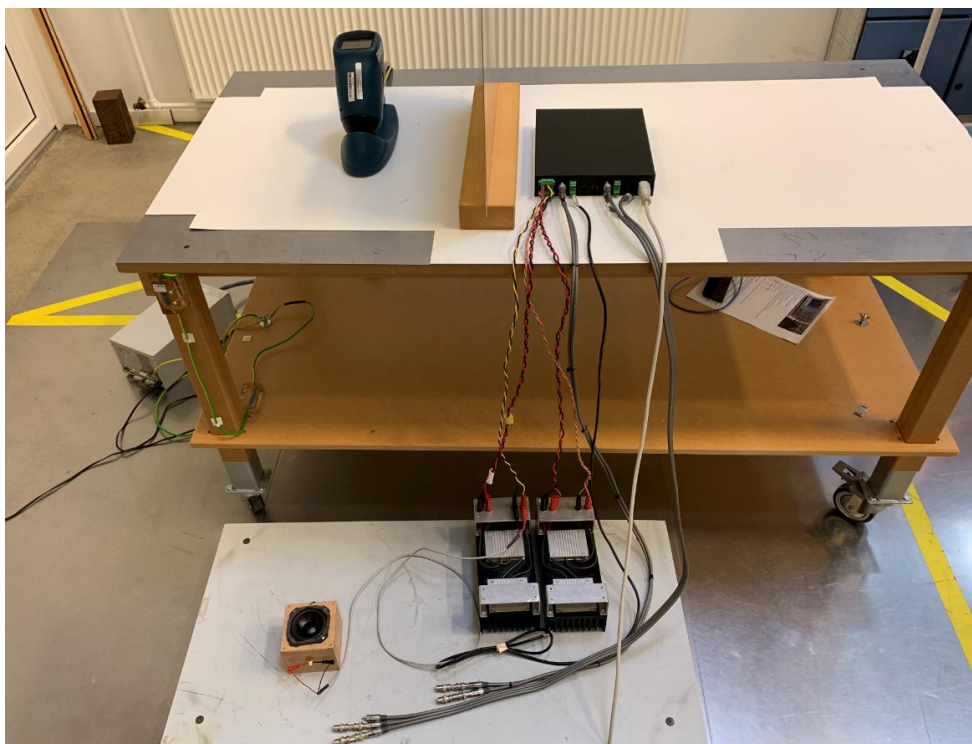
Photo 7. Electrostatic discharge test setup.
