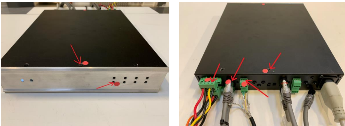
Photo 8. Discharge points for electrostatic discharge tests.
