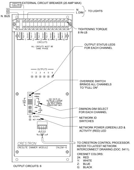
**OUTPUT RATING: 16 AMP PER CIRCUIT**
