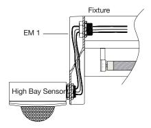
Example of the EM 1 used to mount the HBS 300 high bay occupancy sensor to a fixture. Here, the knockout at the end of the fixture is located greater than 1/2" from the bottom edge of the fixture.
