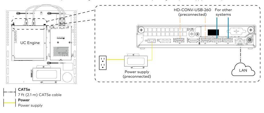
3. Connect displays to the UC Engine.
