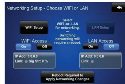
If a static IP address is preferred, from the **WiFi Setup** menu, touch **Set Static IP Address Settings** to display the **WiFi Setup - Static IPs** menu. To stay with DHCP, skip to the bottom of this column to connect to a WiFi access point.
