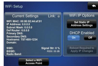
The **WiFi Setup - Static IPs** menu is used to edit **Static IP address**, **Static Subnet Mask**, **Static Default Router**, **Preferred DNS** and **Alternate Preferred DNS** settings. Touch each to display a keypad for entering the new setting.
