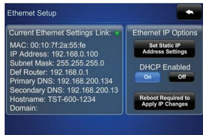
The **Ethernet Setup - Static IPs** menu is used to edit **Static IP address**, **Static Subnet Mask**, **Static Default Router**, **Preferred DNS** and **Alternate Preferred DNS** settings. Touch each to display a keypad for entering the new setting.
