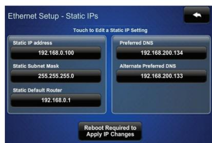
Touch **Reboot Required to Apply IP Changes** to save the new settings and reboot the TST-600.
