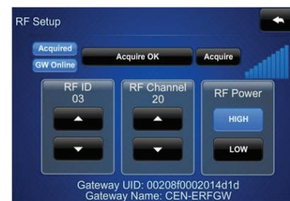
**NOTE:** Select an RF channel between 12 and 23 for maximum range. Channels 11, 24-26 will result in less range but are available if RF interference requires moving the RF channel.
