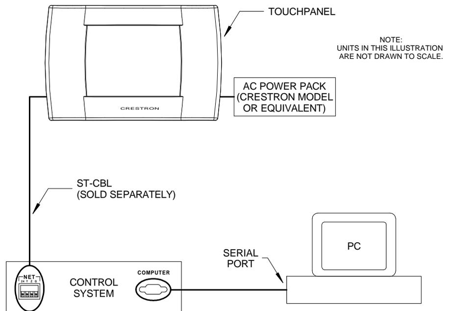
**NOTE:** The cable components in the figure below are part of the SmartTouch Programming Kit (ST-PK). If available, use these components.
