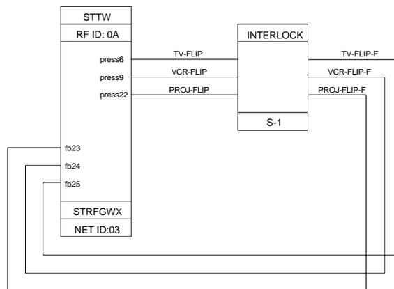
These three signal names should drive an INTERLOCK symbol so that the system can “remember” which page was shown last on the touchpanel. The outputs of the INTERLOCK are assigned unique names: *TV-FLIP-F*, *VCR-FLIP-F*, and *PROJ-FLIP-F*.
