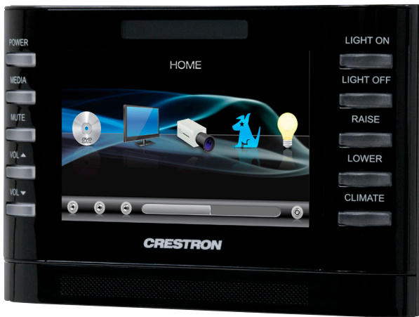
TPMC-4SMD-B-S with WMKU-4SM Universal Wall Mount Kit
