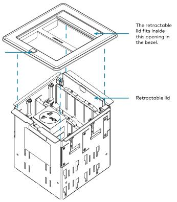
The FT2A-PWR-UN-2 provides two universal AC power receptacles beneath the table (the FT2A-PWR-UN-1-BASIC does not). Use these receptacles to provide power to an electrical FT2 FlipTop assembly and to devices installed below the surface within the FT2 FlipTop assembly
