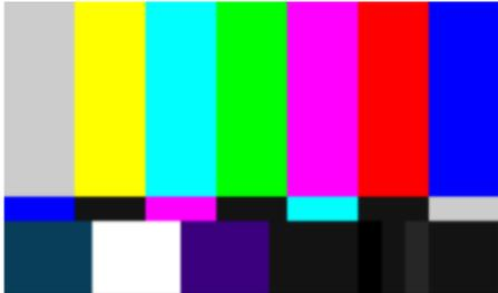
The SMPTE ColorBars test pattern consists of two rows of color bars. The top row contains seven vertical bars of equal height and width, colored from left to right: gray, yellow, cyan, magenta, red, and blue. The bottom row contains seven vertical bars of equal height and width, colored from left to right: blue, black, purple, black, cyan, black, and gray. |
