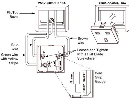
After connecting the wires as shown in the illustration, orient the receptacle as shown and snap the receptacle into the bezel.
