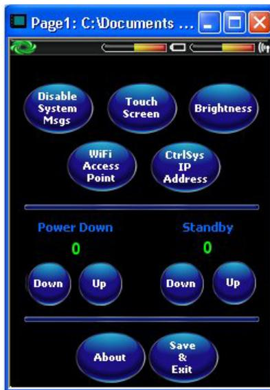
The setup screen enables basic configuration procedures prior to regular operation of the touchpanel.
