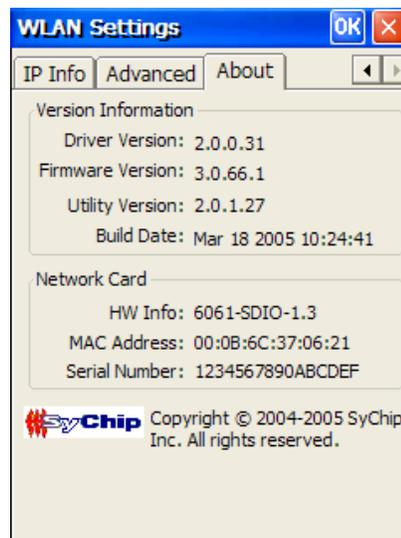
The tab shows version information for the WiFi subsystem of the TPMC-4X. For the overall software version of the TPMC-4X, press the **About** button on the setup screen.
