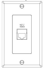
Connect the TPS-4500IMW to the touchpanel using the network/video (10-pin) cable, supplied with touchpanel.
