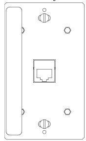
Once the TPS-4500IMW is installed into a 1-gang electrical box, it can be covered with a decora wallplate, purchased separately. Crestron recommends Leviton, part number 80401-\* (where \* denotes an abbreviation that represents color). Refer to the list after this paragraph for available colors at the time of this printing.
