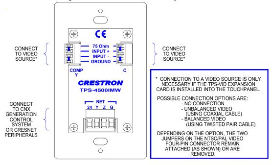
**NOTE:** If there is no video source, do not make connections to either NTSC/PAL video connector. However, leave connector and jumpers attached to the NTSC/PAL video four-pin connector on the TPS-4500IMW.
