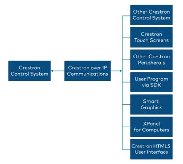
Multiple listeners can be added to the Crestron control system via the user program. Crestron recommends performing a security scan on the control system without a program and then performing the scan again with a program. This will help identify whether any security breaches are created by loading the program.
