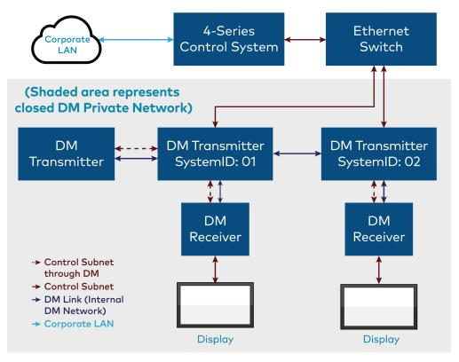
**NOTE:** The SystemID can range from 01 to 64 and must be unique for each DM switcher. By default, the SystemID is set to 01. The ID can be set via the front panel, the SIMPL program, or the System Info tool in Crestron Toolbox. Each DM switcher must be directly connected to the corporate LAN. One DM switcher cannot receive Ethernet via another DM switcher, and each DM switcher must receive an IP address from the control subnet.
