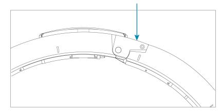
3. To uninstall the speaker, pull the lock tab out to its unlocked (open) position and twist the speaker counterclockwise.
