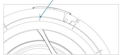
**NOTE:** The lock tab will not lock unless the speaker and bayonet ring indicators fully align.
