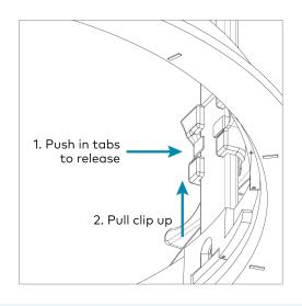
**NOTE:** The length of the bayonet ring rails can be adjusted to match the depth of the mounting hole by manually breaking the additional length off. Make sure the clips are tightened before you do so.
