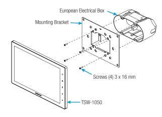
Make connections to the TSW-1050 using Crestron power supplies for Crestron equipment. Power and data connection to the TSW-1050 is provided by a single Ethernet cable connected to the LAN port at the rear of the unit. A Crestron PoE power supply or PoE-capable network switch is recommended (both sold separately). Apply power after the Ethernet cable is connected.
