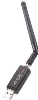
Wi-Spy devices use the Chanalyzer or InSSIDer software to report RF signals. The software can detect other wireless networks as well as 2.4 GHz cordless phones, baby monitors, and microwaves.
