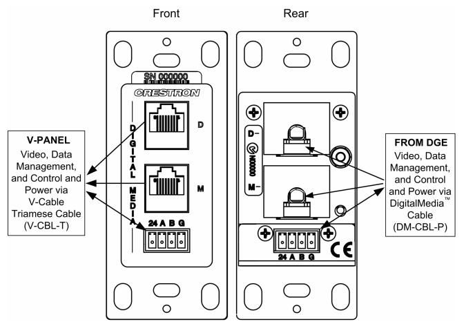
**NOTE:** Ensure the unit is properly grounded by connecting the flying ground wire to an earth ground (building steel).
