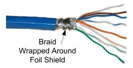
**NOTE:** The braid should wind neatly around the foil shield. Loose braid may cause shorts or difficulty completing assembly of the connector.
