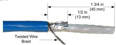
3. Trim the foil shield to 1/2 inch (13 mm) and fold it back against the outer jacket of the cable. Refer to the illustration below.
