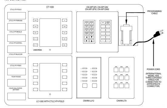
All these interfaces are mounted within a single plastic carry case (14"L x 18"W x 4.5"H). Simply open the case, plug the power cord into a grounded outlet, and begin using the interfaces. A program has been preloaded into the kit for the user's convenience. The kit also contains a programming cable if the user decides to replace the preloaded program. Consult a customer service representative if unsure on how to program the kit.
