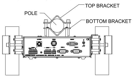
1. Mount the bottom bracket of the MK-QM-RMCRX to the QM-RMCRX PEM nuts using the four #6-32 screws and spacers provided.
