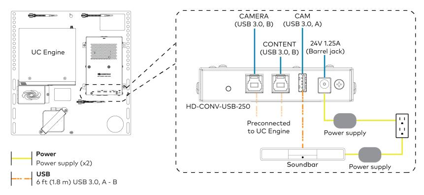
3. Connect power, the content ingest device (HD-CONV-USB-250), and LAN to the top of the UC Presentation Transmitter.
