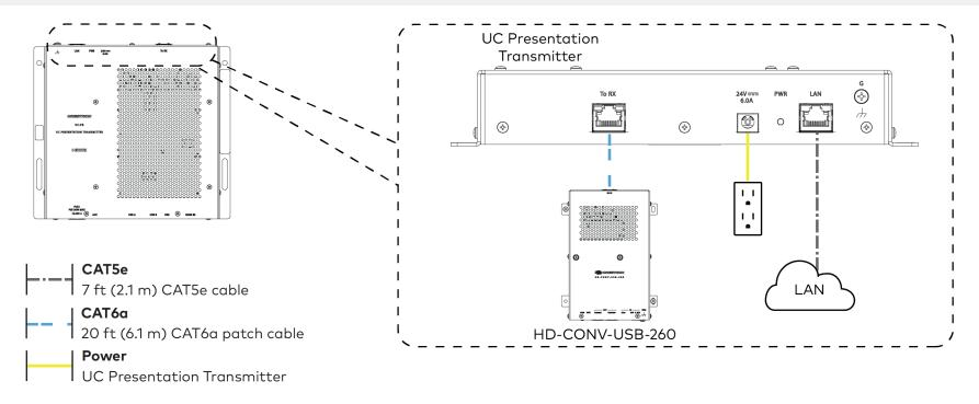
5. Connect the touch screen to the bottom of the UC Presentation Transmitter.
