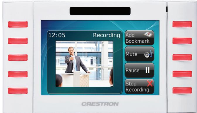
**NOTE:** The CAPTURE-HD records camera video via the composite or SDI input, not via streaming MJPEG video. The MJPEG video stream is only used for preview on the CAPTURE-TPMC-4SM touch screen. The Crestron CAM-IBF-100 and CAM-IPTZ-101 cameras can output both composite and MJPEG streams simultaneously. If using a third-party camera, be sure to check its video output capabilities if touch screen preview is desired.
