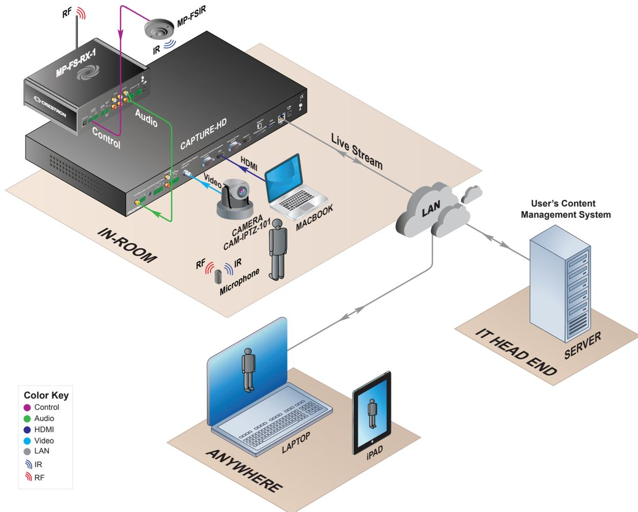
The illustration above shows how the CAPTURE-HD may be used with a Content Management System (CMS). In this configuration the CAPTURE-HD provides live content, which can be recorded, edited, and processed:
