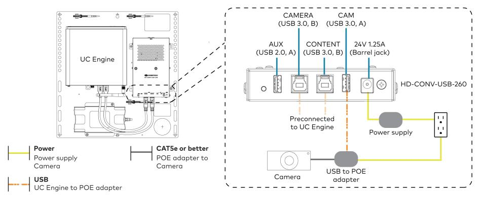
4. Bundle the cables to the bracket assembly with the integrated cable tie wraps. The cable tie wraps are reusable.
