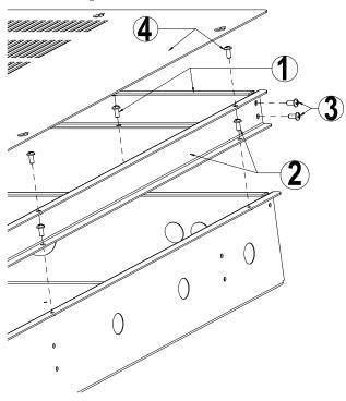
1. As shown in the installation diagram, place a horizontal pan on the bottom and top of the CAEN enclosure (edges facing inward). Use a #2 Phillips tip screwdriver to secure the horizontal pans to the enclosure using the 8-32 screws.
