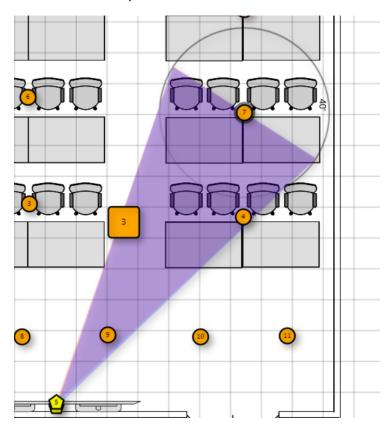
Five Virtual Mics are placed along the presentation area in the front of each space of the divisible room. This ensures that whenever audio is detected in the presentation area, the AutoTracker camera at the back of the room switches to the presenter.
