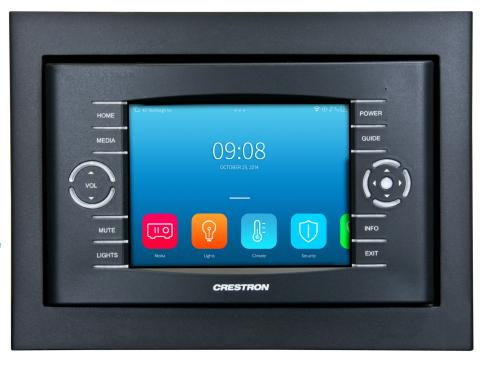
the convenience of a stationary wall mount touch screen while docked, with the ability to go mobile at the press of a button.
