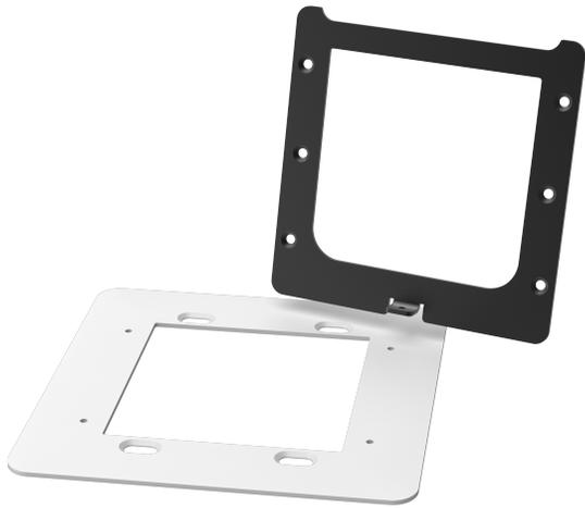
The TSS-470E-RMB-2G retrofit mounting bracket is used to mount a [TSS-470E-B-T](#) desk scheduling touch screen over a flush wall-mounted 2-gang U.S. electrical box. The TSS-470E-RMB-2G is ideal for applications that require low voltage termination in an in-wall electrical box near a reservable space. A security screw is also provided to prevent unauthorized removal of the touch screen from the mounting bracket.
