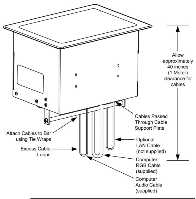
**NOTE:** Ensure that the cables have sufficient clearance to enable smooth movement. Allow approximately 40 inches (1 meter) from the top surface of the FlipTop box.
