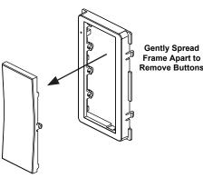
3. Insert new buttons through the front of the bezel and snap into place as shown in the following diagram. Ensure that the LED strip is on the left side.
