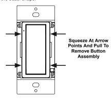
Remove button(s) from the front of the button assembly as shown in the following diagram.
