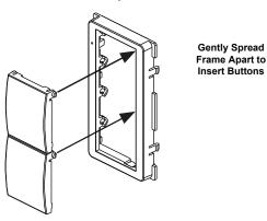
4. Attach button assembly to the device as shown in the following diagram. Ensure that LED strip is on the left side.
