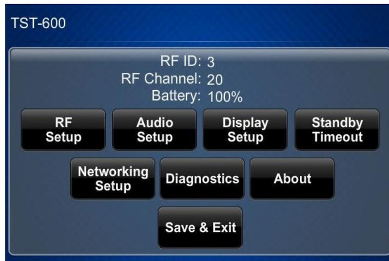
The main menu displays the current *RF ID*, *RF Channel* and battery status and is also comprised of buttons for **RF Setup**, **Audio Setup**, **Display Setup**, **Standby Timeout**, **Networking Setup**, and **Diagnostics**. In addition, there are buttons that provide information about the touch screen and a **Save & Exit** button. The functions of each are detailed in the next section of this guide.
