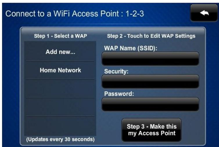
The left side of the “Connect to a WiFi Access Point: 1-2-3” menu displays a list of available access points. Touch the name of the desired access point.
