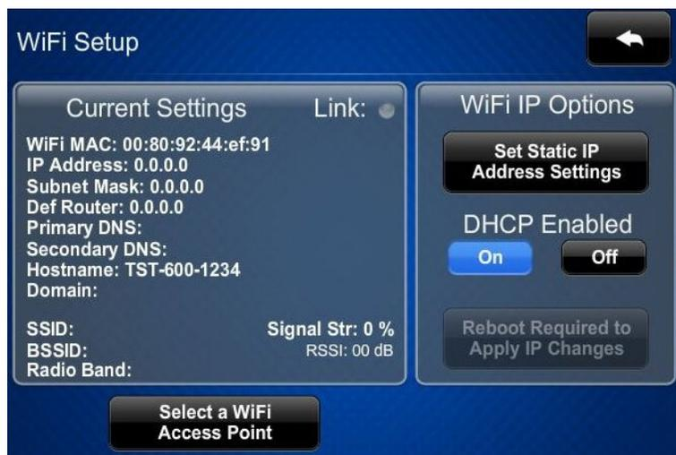
If a static IP address is preferred, from the “WiFi Setup” menu, touch **Set Static IP Address Settings** to display the “WiFi Setup – Static IPs” menu.
