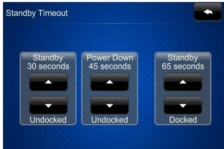
The “Standby Timeout” screen provides controls to adjust *Standby* timeout (from 0 to 120 seconds) and the *Power Down* timeout (from 0 to 240 seconds), both for when
