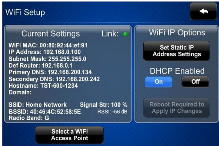
From the “WiFi Setup” menu, touch **Select a WiFi Access Point** to display the “Connect to a WiFi Access Point: 1-2-3” menu.
