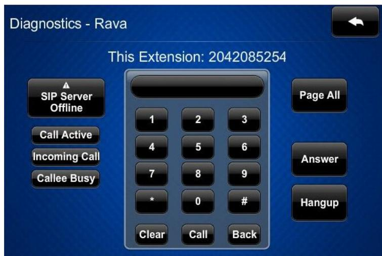
The “Diagnostics - Rava” screen provides controls for testing the use of Crestron’s Rava® SIP Intercom with the TST-600. It can be used to call another Rava-capable touch screen and to test projects and settings. To place a call, dial the extension of the desired touch screen and press **Call**. If the intercom works but the project does not, there is an issue with the project; if the intercom does not work, there is an issue with the settings.
