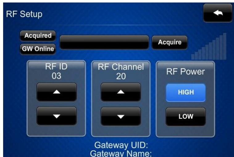
The “RF Setup” screen has *Acquired* and *GW Online* indicators to show the status of the TST-600 and associated gateway. To the right of these is a message display area used to show the status of acquire processes, an **Acquire** button used to initiate acquires and a bar graph showing RF signal strength. Below these are controls for setting the *RF ID*, *RF Channel*, and *RF Power*. At the bottom of the screen, the *Gateway UID* and *Gateway Name* are displayed.
