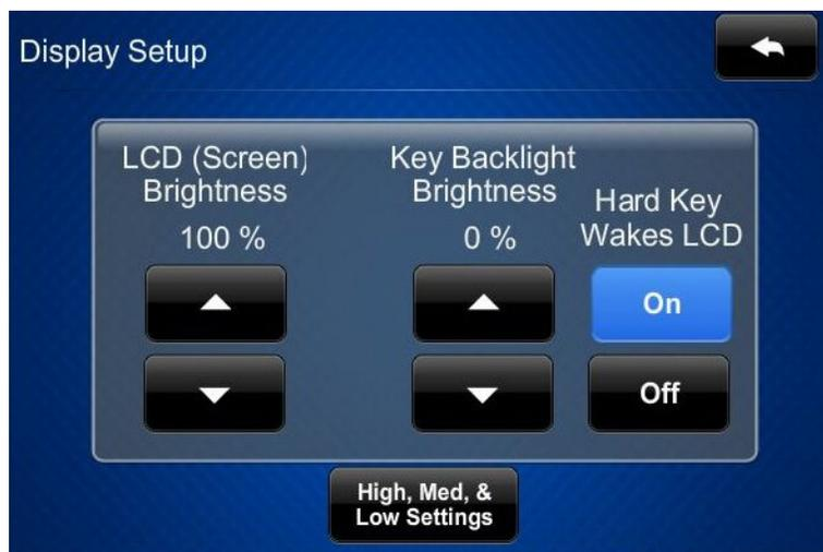
The “Display Setup” menu provides controls for *LCD (Screen) Brightness*, *Key Backlight Brightness*, and **On** and **Off** controls for *Hard Key Wakes LCD*.
