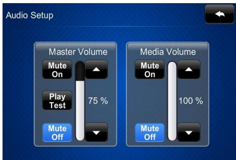
The “Audio Setup” screen provides controls for muting (or unmuting) the audio, adjusting level for both *Master Volume* and *Media Volume*, as well as a control for playing a test audio file. The *Media Volume* controls adjust H.264 streaming media level in relation to the *Master Volume* controls.
