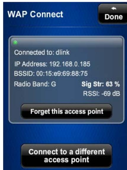
8. Tap **Done** to accept the connection to the wireless access point and to display the **WiFi Setup** screen.
