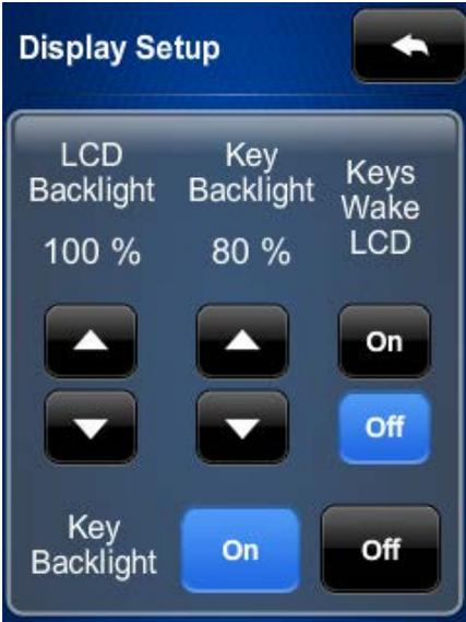
The **Display Setup** screen provides brightness controls for **LCD Backlight** and **Key Backlight**, and **On** and **Off** controls for **Keys Wake LCD** and **Key Backlight**.
