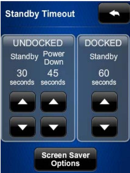
The **Standby Timeout** screen provides controls to adjust the **Standby** timeout (from 0 to 120 seconds) and the **Power Down** timeout (from 0 to 240 seconds) for when the TSR-302 is undocked. There is also a **Standby** timeout control (from 0 to 120 seconds) for when the TSR-302 is docked.
