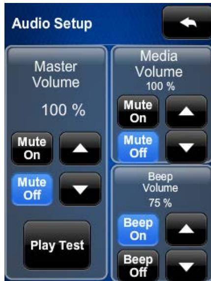
The **Audio Setup** screen provides controls for muting (or unmuting) the audio, adjusting the **Master Volume** and the **Media Volume**, and playing a test audio file. The **Media Volume** controls adjust H.264 streaming media level in relation to the **Master Volume** controls. The **Beep Volume** controls adjust the level at which key click sounds (if enabled) will play when a button is pressed.
