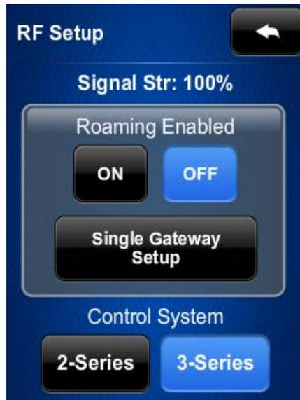
The **RF Setup** screen shows the RF signal strength and has controls for enabling or disabling roaming.
