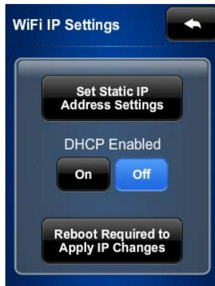
11. Tap **Set Static IP Address Settings** to display the **Static IPs** screen.
