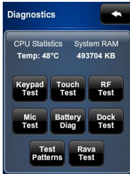
The **Diagnostics** screen displays the CPU temperature and the system RAM. It also contains controls to run a **Keypad Test**, **Touch Test**, **RF Test**, **Mic Test**, **Dock Test**, and **Rava Test**. In addition, there are controls to examine the battery condition and to open various test pattern screens.
