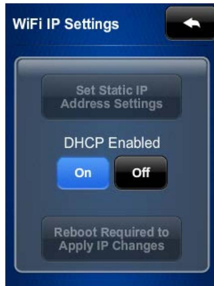
10. The TSR-302 ships with DHCP enabled by default. To use DHCP, tap
