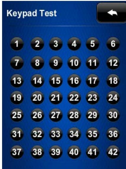
The **Keypad Test** screen contains 42 indicators that correspond to the 42 buttons on the TSR-302. The appropriate indicator lights to confirm operation of each pressed button.
