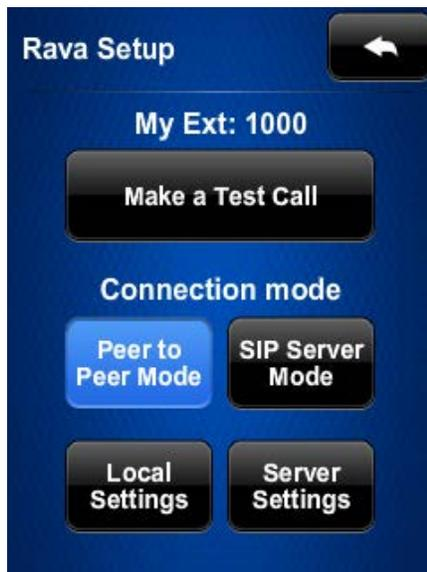
The **Rava Setup** screen provides controls for testing the use of Crestron's Rava® SIP Intercom with the TSR-302. Use this screen to configure the TSR-302 to make peer calls to
