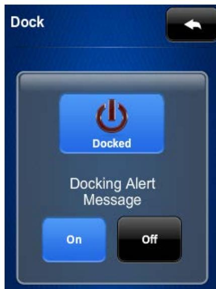
The **Dock** screen has an indicator to confirm that the TSR-302 is docked. The **On** and **Off** buttons enable or disable the dock alert message and the chime that sounds when the TSR-302 is docked.
