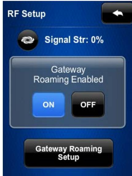
Tap **Gateway Roaming Setup** to display the **RF Roaming Setup** screen.
