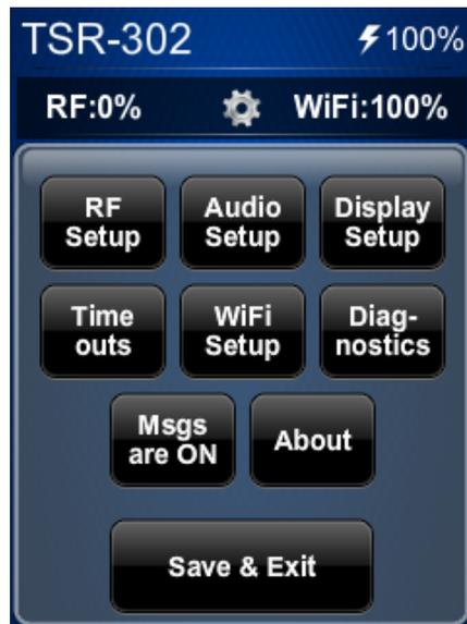
The main menu displays the current battery status, gateway (RF) signal strength, and Wi-Fi® signal strength, as well as **RF Setup**, **Audio Setup**, **Display Setup**, **Timeouts**, **WiFi Setup**, and **Diagnostics** buttons. In addition, there is a button that toggles on-screen messages on and off, a button that provides information about the TSR-302, and a **Save & Exit** button. The functions of each are detailed in the next section of this guide.
