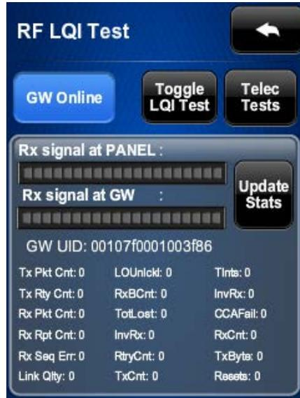
The **RF LQI Test** screen provides diagnostic information about the signals from the gateway.
