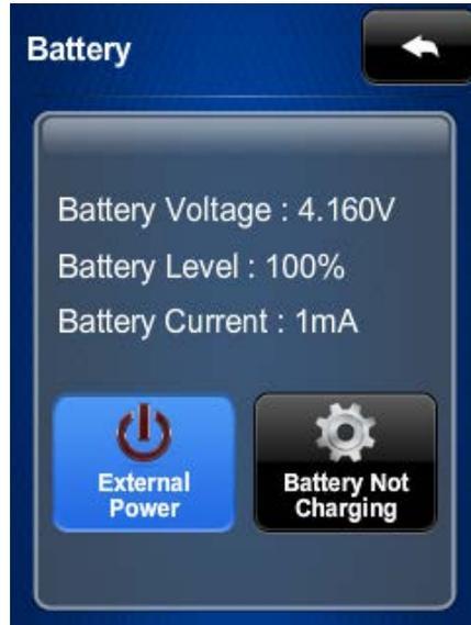
The **Battery** screen provides information about the battery condition and also has an indicator to show when external power is being applied.
