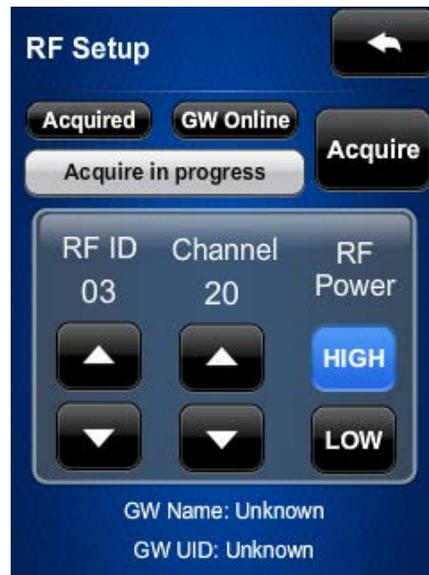
3. When the process is complete, the screen displays an “Acquire OK” message. Press **ACQUIRE** on the gateway to exit Acquire mode. The LED turns off.
