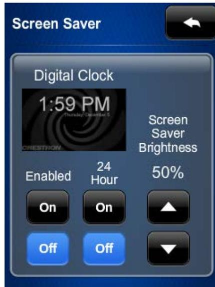
This screen has **On** and **Off** controls for the screen saver and for displaying the time in a 24-hour format. In addition, there are **Screen Saver Brightness** controls.
