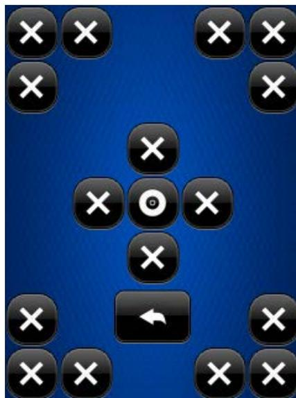
The touch test screen contains indicators that light when the corresponding section of the touch screen on the device is tapped.
