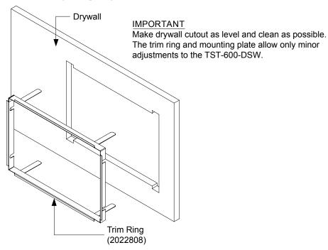
**NOTE:** The required TST-600-DSW-PMK or TST-600-DSW-BB is not shown.
