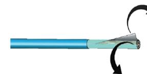
3. Fold back the drain wire and wrap it around the foil shield.
