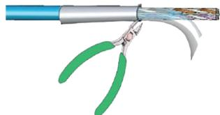
5. Gently spread the four twisted pairs to expose the center spline.
