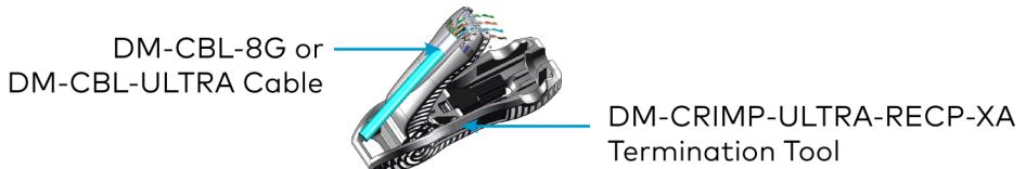
3. Insert the wires of the DM-CBL-8G or the DM-CBL-ULTRA into the termination module, following the guide printed on the tool for correct wire placement.
