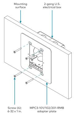
2. Use the two included  $4-40 \times 1/2$  in. screws to attach the MPC3 mounting plate (included with the MPC3 device) and the included metal cover to the adapter plate. The MPC3-201 mounting plate is shown in the illustration below as an example.
