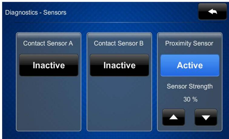
The **Diagnostics - Sensors** screen can be used to view the status of the built-in proximity sensor or any sensors attached to the TSW-732. This screen also provides controls for adjusting the proximity sensor strength.
