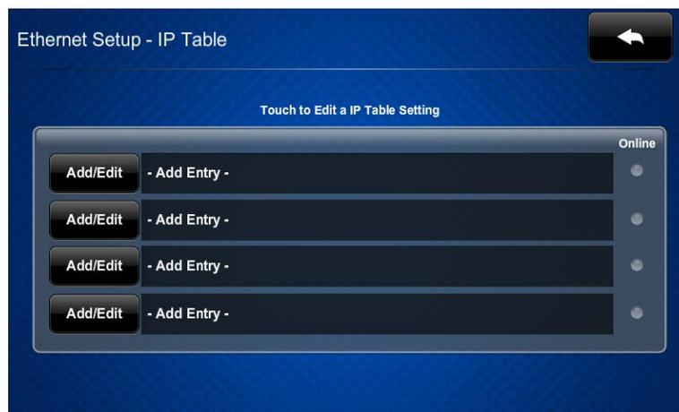
The **Ethernet Setup - IP Table** screen displays up to four IP table settings, each of which has an **Online** indicator. To add or edit an entry, tap the **Add/Edit** button to its left. The **Ethernet Setup - Edit IP Table Entry** screen is displayed.
