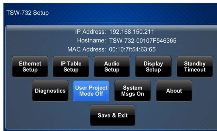
The TSW-732 Setup screen is composed of buttons for Ethernet setup, IP table setup, audio setup, display setup, standby timeout, and diagnostics. In addition, there are buttons to toggle user project mode and system messages on or off. An **About** button provides information about the touch screen, and a **Save & Exit** button saves settings and exits the setup screens. The functions of each are detailed in the following pages of this guide.
