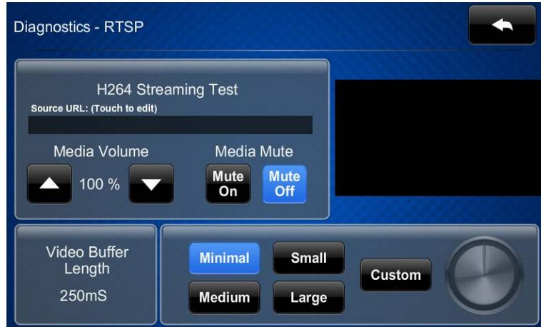
The **Diagnostics - RTSP** screen is used to test whether Real Time Streaming Protocol is functioning on the touch screen. Tap the area below **Source URL: (Touch to edit)** to open the on-screen keyboard. Enter the URL for an H.264 video and then tap **Save**. The video is displayed on the right side of the **Diagnostics - RTSP** screen. The bottom part of the screen provides controls to select among video buffer lengths or to select a custom length adjustable via a virtual knob.
