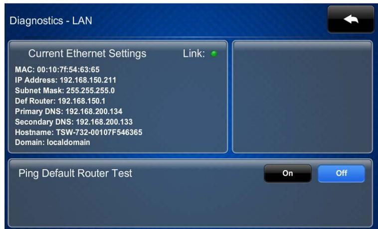
The **Diagnostics - LAN** screen displays the touch screen's MAC and IP addresses, subnet mask, default router, primary and secondary DNS, hostname, and domain. This screen also contains a Link indicator to show the status of the Ethernet connection and controls to test the connection to the default router.
