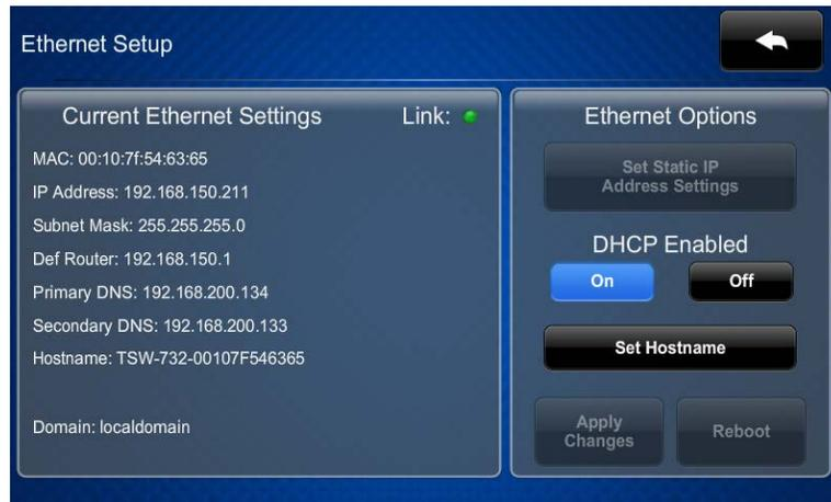
The **Ethernet Setup** screen displays the TSW-732's MAC and IP addresses, subnet mask, default router, primary and secondary DNS, hostname, and domain. There are controls for turning DHCP on and off. When DHCP is off, a **Set Static IP Address Settings** button provides access to controls that allow editing of these settings. This screen also contains a link indicator to show the status of the Ethernet connection.
