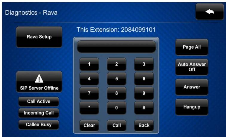
The **Diagnostics - Rava** screen provides controls for testing the use of the Rava® SIP Intercom with the TSW-732. It can be used to call another Rava-capable touch screen and to test projects and settings. To place a call, dial the extension of the desired touch screen and tap **Call**. If the intercom works but the project does not, there is an issue with the project; if the intercom does not work, there is an issue with the settings.
