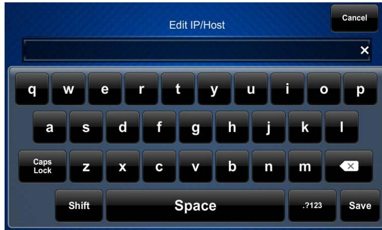
Use the keyboard to make the new entry. Tap **Cancel** to return to the **Ethernet Setup - Edit IP Table Entry** screen. Tap the "x" in the text field to clear any previous entry. Tap
