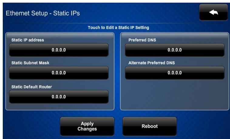
To edit the static IP address, static subnet mask, static default router, preferred DNS, or alternate preferred DNS, tap the button directly under the label for the entry. The on-screen numeric keypad opens.
