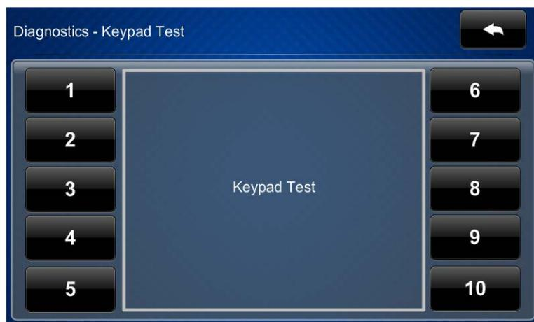
The **Diagnostics - Keypad Test** screen can be used to test the function of the hard keys. When a hard key is pressed, its corresponding indicator on the screen lights.
