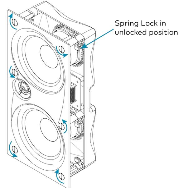
3. To remove the speaker, turn the Spring Lock releases 90° in the opposite direction of the arrows indicated. The Spring Locks will return to their unlocked position.
