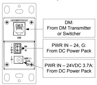
**CAUTION:** The V24-IMCW-C can be powered via the **24** G 2-pin connection on the rear of the unit or the **24VDC 3.7A** jacks on either the front or the rear of the unit. To avoid possible damage to the unit, use only one of these connectors.
