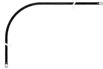
90° Degree Bend and 20 in Minimum Bend Radius
