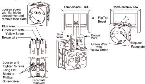
After connecting the wires as shown in the illustration, replace the faceplate, orient the receptacle as shown and snap the receptacle into the bezel.
