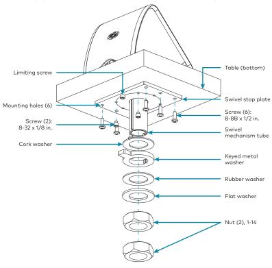
4. Tighten and adjust the upper 1-14 nut onto the swivel tube to achieve the desired resistance in the swivel assembly motion.
