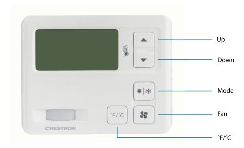
To enter Setup mode, press and hold the **Down** button. While holding the **Down** button, simultaneously press and hold the **Mode** and **Fan** buttons until the **SETUP: SYSTEM** screen is displayed.
