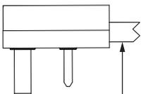
Low-profile power cord must clear top of FT2 series bezel
