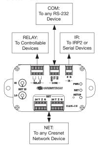
**CAUTION**: Incorrect wiring may damage the C2N-IO.
